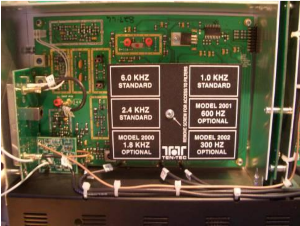
Figure A-3: Modified 9 MHz IF board with Z10000 Buffer at lower left (Photo Courtesy of Grant Bright, W4OJC)
