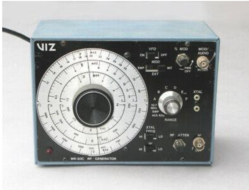
Figure 5 : The VIZ WR-50C is typical of low cost entry-level RF signal generators. Additional features here included a scanning function for IF alignment at 455kHz and 10.7MHz and a crystal checking function.
