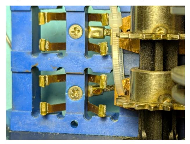
New brushes were needed. However, by this time SteppIR EHU parts were no longer available! So I decided to salvage the existing parts. The brushes were gently ground down with a sharpening stone and polished with 2000 Grit Wet/Dry paper. The tapes were then fully extended and wiped down with 99% isopropyl alcohol. With the tapes rewound, the brushes were given a final alcohol cleaning before sealing up the driven element EHU.
