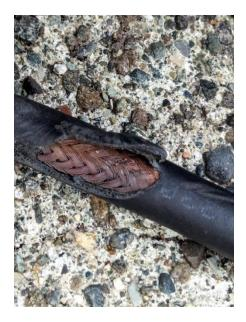
While removing the fibreglass tubes from the EHUs I encountered an additional problem. The 6 flexible couplings that secure the 6 element tubes to the EHUs had begun to split. These couplings had been covered with PVC tape to protect them from UV but they still had deteriorated badly.
