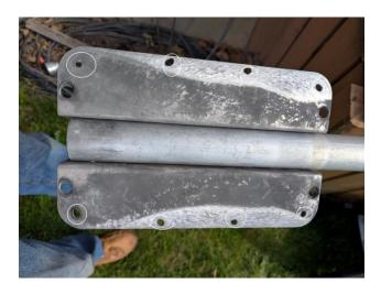
In an effort to reduce this type of movement as well as eliminate flex in the housing I fabricated a base reinforcement of 3/16th inch aluminum. To distribute the load across the mounting screws and the fibreglass EHU cover a top rail of  $1/16^{th}$  x 1 inch aluminum angle was also added.
